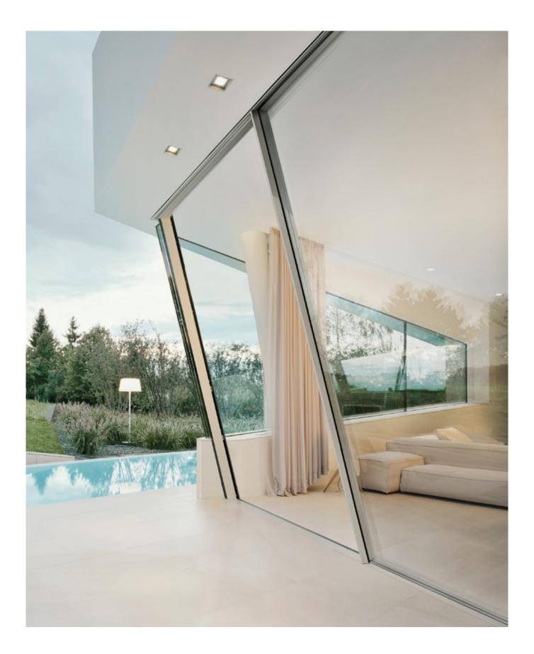
Sky-Frame Slope sliding windows can either extend into the room or project outwards from the facade at an angle of up to 20°. The system meets all Sky-Frame standards while generating a distinctive spatial geometry. The bearing assembly is able to accommodate all vertical and horizontal forces, thereby achieving superior running performance. Regardless of the direction of the window, the drainage system meets all requirements for driving rain resistance.
